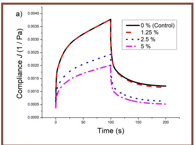
Figure a): Creep-recovery curves for gluten, with different levels of coffee cherry pulp powder (CCPP) substitution. Graphs plotted with averages of Kelvin-Voigt model.
