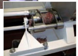
Pictured is the complete grinder with a close-up of the spring cutter mechanism in operation.
