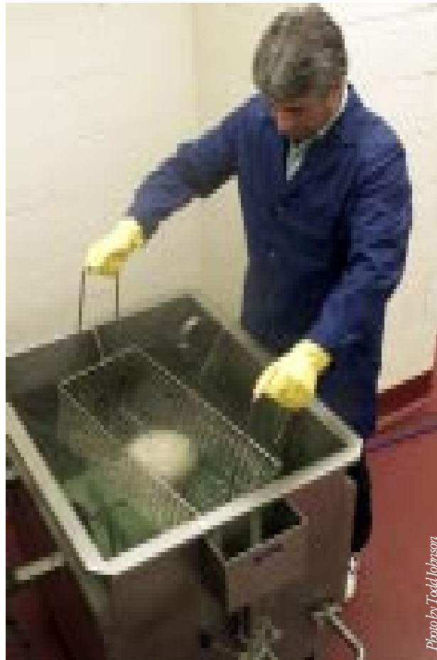
FAPC microbiologist, Peter Muriana, uses Unitherm's process to evaluate the effects of post-package pasteurization on Listeria monocytogenes inoculated turkey product.
