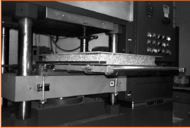
Value-added processing provides a new market for previously non-marketable Eastern red cedar. Production of one- and three-layer particle board utilizes the entire tree, giving landowners an outlet for the bothersome plant.
