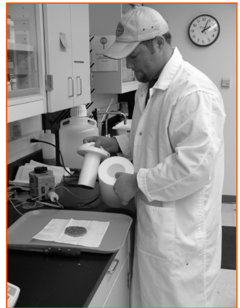
Ohmic heating is a direct-heating method capable of rapidly cooking foods by passing electrical current through the product.
