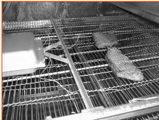
A six-channel data logger passes through an oven to record actual cooking temperatures.
